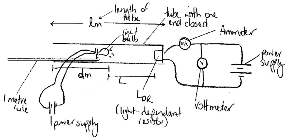
(a) Set up the experiment as shown above. Measure the distance between the LDR and the light bulb  $L = (l - d)$  m in the above experiment. At this distance, <sup>note</sup> measure the current recorded and the voltage recorded. Repeat the experiment by varying the length of  $d$  (to obtain varying distance between light bulb and the LDR) then record the current and voltage <sup>with</sup> different distance  $L$ .
