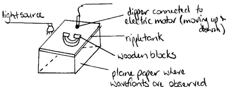
A ripple tank is set up as shown. When wave pass to the small gap they are diffracted. [3]
