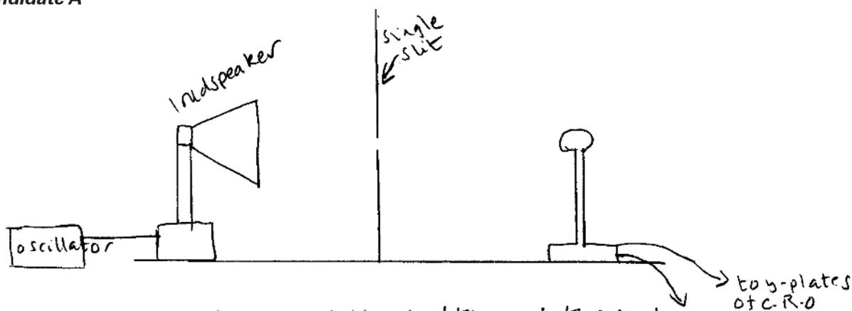
the sound wave is diffracted through the single slit and the C.R.O records pulses of waves with varying intensities. [3]
